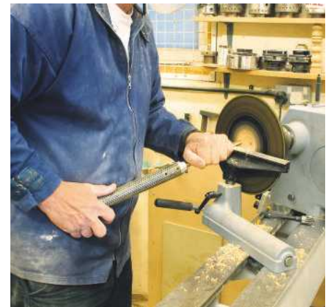
▲ Pic.24 When hallowing tuck the tool into your side so you can move your body around easily. The hand-over grip allows the tool to slide through Les's hands as the tool advances
